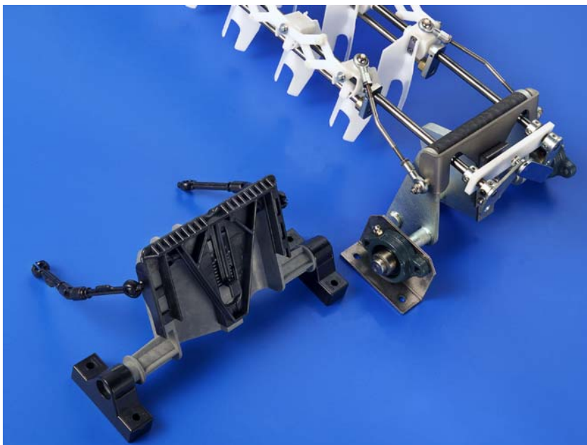
The pivot block (lower left) consists of five distinct molded parts with a part reduction of 120 pieces per packing machine and time for machining, welding and assembly all eliminated.
